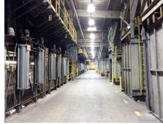
Their in-house designed and developed bottom-drop furnaces allow the castings to move from the furnace to the quench tank in under seven seconds.
