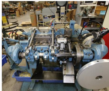
**\*\*Fourslide stamping process saves on material cost by ordering material true to part.**
